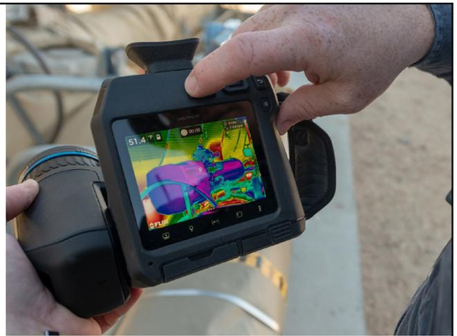
*Images and videos from OGI devices such as the FLIR GF77 can provide a fact-base for troubleshooting safety and operations issues.*
